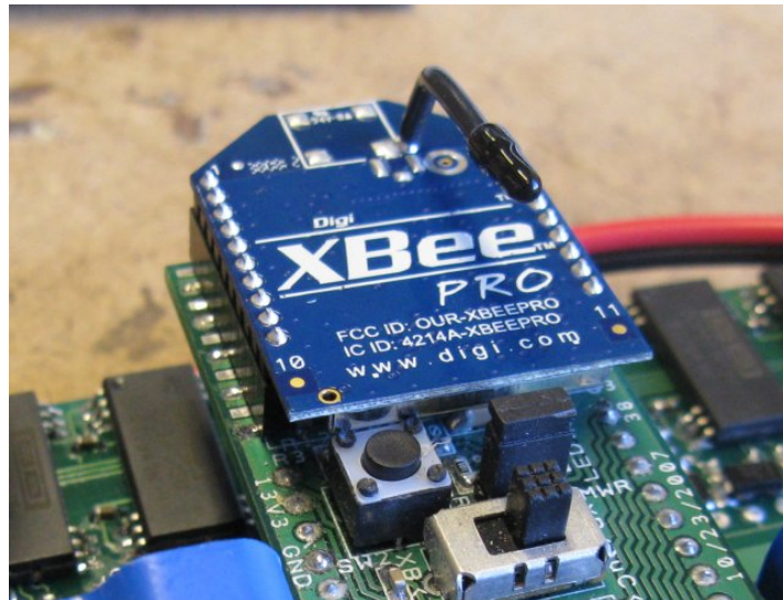
Figure 69: The 2.4GHz transceiver integrated into the case study motor controller.
