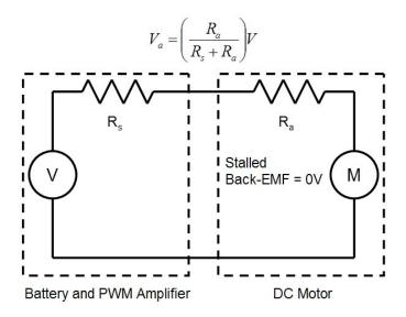
Figure 16: The simplified electrical schematic of a stalled DC motor with a fixed supply voltage. The source impedance of the supply causes a division of the armature voltage and limits the stall current of the motor.
