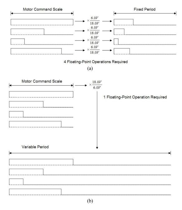
Figure 11: The method of scaling motor commands to account for battery voltages above the highest rated motor voltage. Fixed-frequency operation (a) has been replaced by variable-frequency operation (b) to minimize the computation required.
