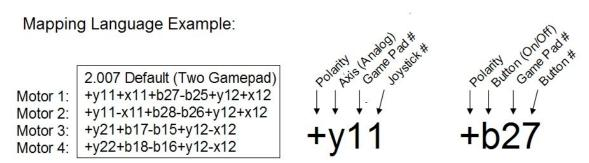
Figure 13: An example of the mapping language used by the host computer to easily configure the mapping of input devices to motor commands. The user can edit a text file with control mappings to change motor polarities, modify existing mappings, or create new mappings from scratch. The example shown is the default 2.007 control scheme.
