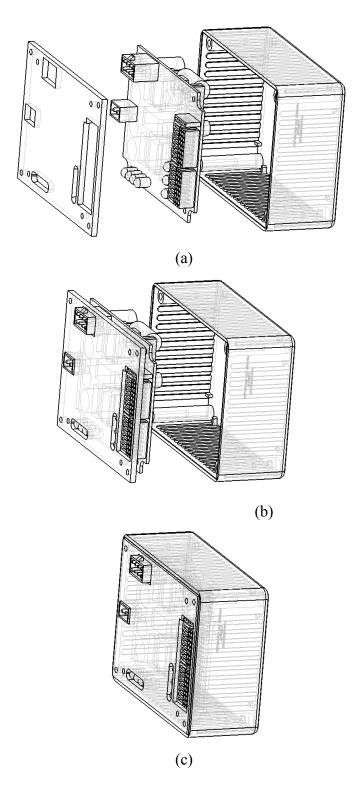
Figure 3: The control box is designed for easy single-axis assembly. The three main components (cover, board, and box) are shown expanded (a). The board and cover are attached to each other first (b), then the cover and board are both secured to the box to complete the assembly (c).
