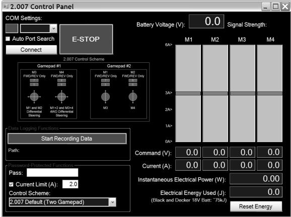
Figure 12: The graphic user interface displayed on-screen at the host PC is designed to give the robot driver feedback on machine performance.
