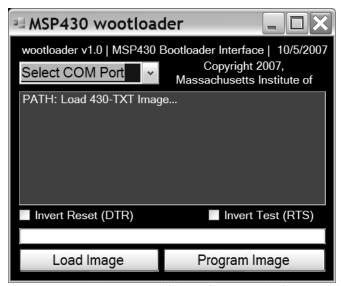
Figure 14: The wireless bootloader ("wootloader") interface. Despite its name, it may be used either with a wired (USB) or wireless (ZigBee) serial connection.
