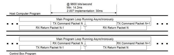
Figure 8: Asynchronous data transmission and reception allows for overlapping program loops and efficient program execution that is never in a "waiting" state.
