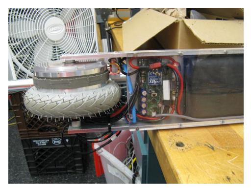
Figure 38: The rear wheel, motor, and motor drive of Pneu Scooter.
