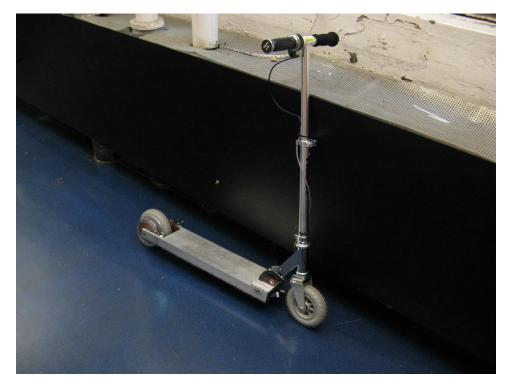
Figure 37: Pneu Scooter, a lightweight electric kick-scooter with a custom in-wheel motor.
